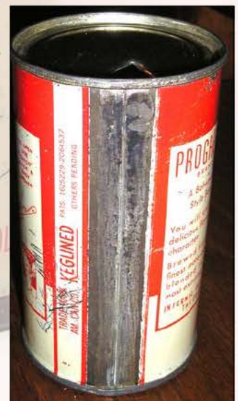
After the tin and solder patch, it was then blended to match the rest of the seam.
