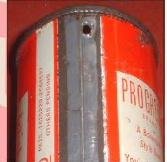
This is the can upon arrival with a hole punched through the top of the seam.
