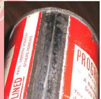
After the tin and solder patch, it was then blended to match the rest of the seam.
